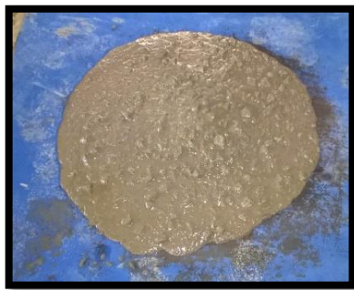
Variation of Plastic aggregate on Slump flow
